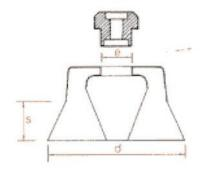
According to above drawing, 5" diameter, 1.1/8" trim length. Total N° of .020" wire ends in the brush: 3,960 Weight of total product: 870 gr.
