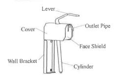
1. Loosen screws and slide aluminum cover forward until it stops against the screws. This action should release the wall bracket, which can be removed by holding on to the cover and pulling the wall bracket downward.
