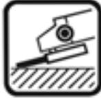
The best results are achieved with an angle of 30° to 40° for grinding. Move the tool back and forth with light pressure. In this manner, the workpiece does not become too hot, discoloration will not occur, and no ridges are produced.
